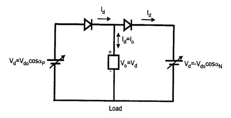
The input and output voltages are adjusted to be equal and the load current can flow in either direction. Thus,
