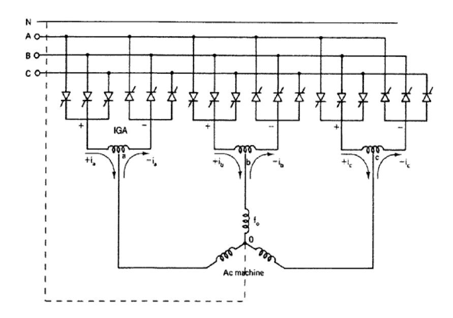
Each phase group functions as a dual converter but the firing angle of each group is modulated sinusoidally with  $2\pi/3$  phase angle shift ->  $3\Phi$  balanced voltage at the motor terminal. An inter-group reactor (IGR) is connected to each phase to restrict circulating current. An output phase wave is achieved by sinusoidal modulation of the thyristor firing angles.
