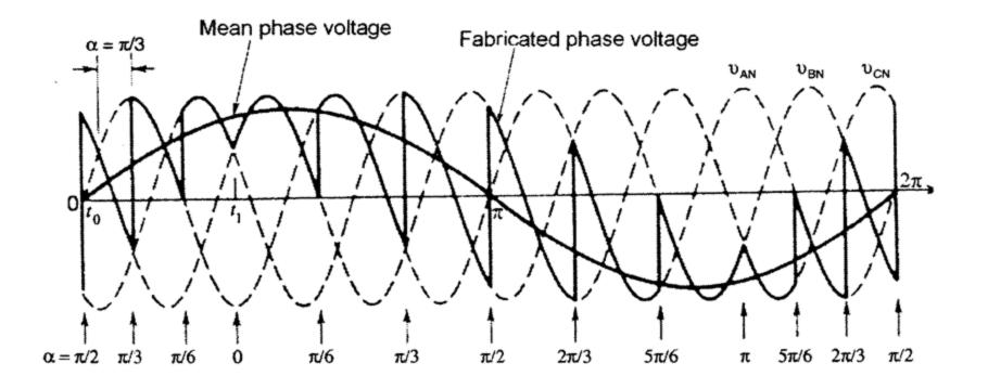
A variable voltage, variable frequency motor drive signal can be achieved by adjusting the modulation depth and output frequency of the converter.
